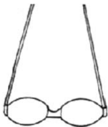
Incorrect Temples are too close together
